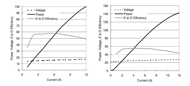
**Figure 2.** (Left) A Pearl module producing over 80 W of optical power coupled into a 200  $\mu$ m fiber. The power per unit volume for this module is approximately 0.95 W/cm<sup>3</sup>. (Right) A high-power Pearl module with an output over 120 W of power also coupled into a 200  $\mu$ m fiber. The power per unit volume for this module is approximately 0.93 W/cm<sup>3</sup>. Both of these devices are designed at 976 nm, and have a spectral FWHM smaller than 3.5 nm.
