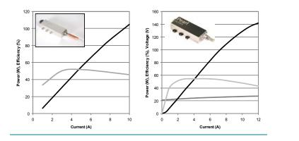
*Figure 3.* (*left*) A Pearl module capable of coupling over 100W of optical power into a 0.15 NA, 105um fiber. (right) A Pearl module capable of coupling over 120W into a 200um, 0.2 NA fiber.
