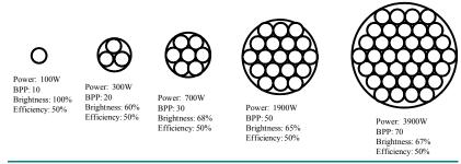
**Figure 7.** An illustration of the power and BPP of 1, 3, 7, 19, and 39 element fiber bundles. As can be seen, about 65% of the brightness is preserved when using fiber bundles. The residual brightness loss can be attributed to the interstitial space between fibers, as well as the thickness of the cladding layers. Note that efficiency values of approximately 50% are achieved for all power levels, proving a method to scale power without losing efficiency.
