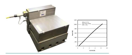
**Figure 6.** (left) A KW-class laser diode system based on single emitters. The device utilizes wavelength beam combination to achieve over 1000 W of output power into a 400um, 0.2 NA fiber. (right) The light versus current curve for the module.
