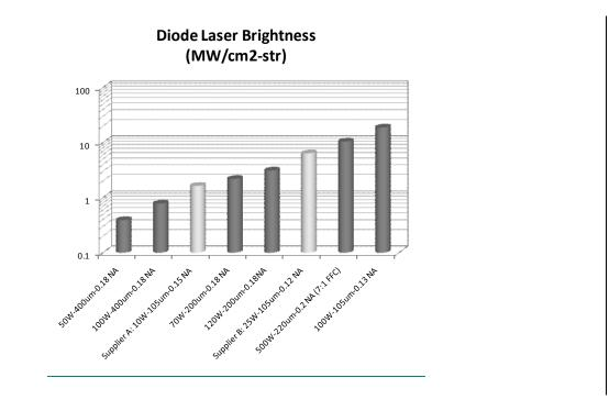
*Figure 2.* Diode laser brightness (MW/cm2-str) for various diode laser pump modules. Brightness levels in excess of 18  $MW/cm^2$ -str have been achieved using nLIGHT's Pearl<sup>TM</sup> product line.
