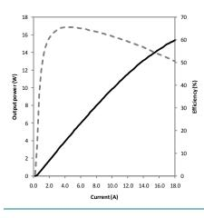
*Figure 1.* LI and efficiency curves for a single emitter diode laser developed at nLIGHT. Such a device is rated at 10W of optical power with an operating efficiency of over 60% and a FIT rate of 1200 (90% confidence level).
