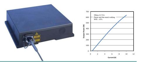
*Figure 5.* (*left*) A picture of the single emitter-based system. The device utilizes a single polarization and wavelength to put over 500 W of output power into a 300um, 0.2 NA fiber. (right) The light versus current curve for the module.
