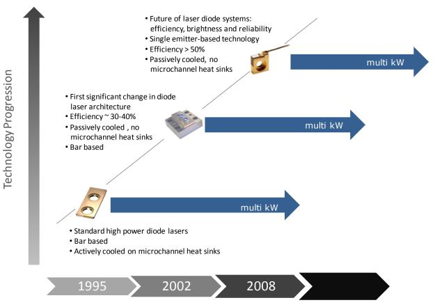
Figure 4: Technology progression of laser diode systems. The move to single emitter-based diode lasers simultaneously improves brightness and efficiency from the diode laser system.
