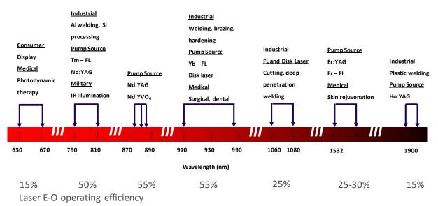
Figure 3: Wavelength requirements for industrial, pumping, medical, and consumer applications with laser electrical-tooptical efficiency.
