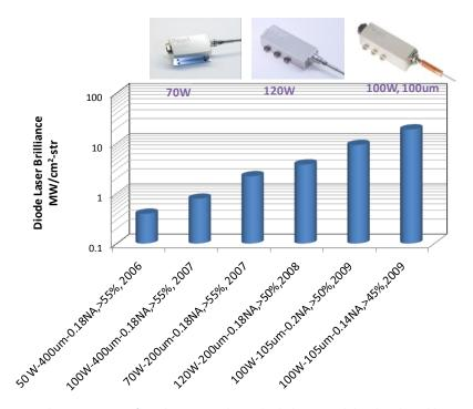
Figure 5: Brilliance scaling over time of single-emitter direct diode laser modules developed by nLIGHT Photonics.
