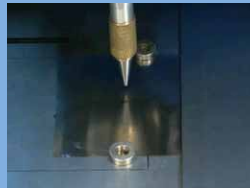
Thin stainless cutting: Fiber laser 90W, 40um
