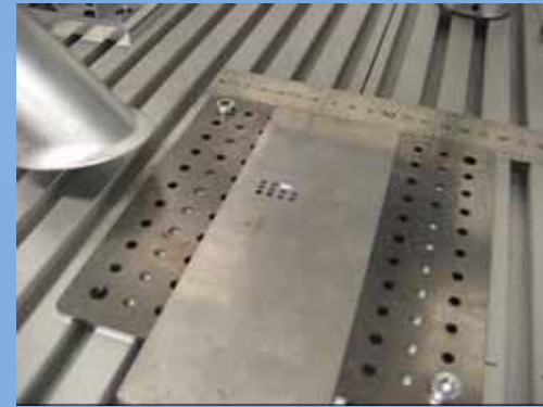
Marking: Fiber laser 25...50W, 80um
