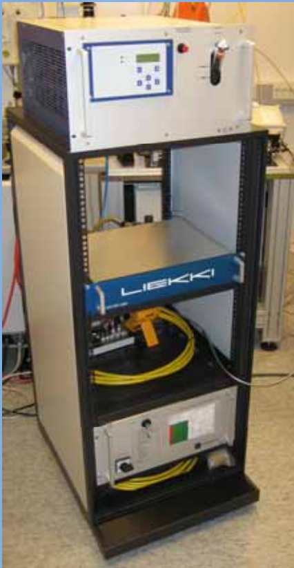
Liekki OE-Yb-RML-400 "Beam converter" system with Laserline diodelaser and chiller
