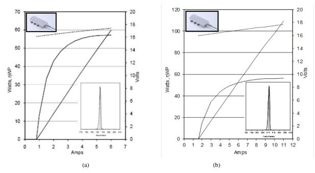
Figure 9: LIV and spectrum from (a) 200 μm 0.18 NA 792 nm fiber-coupled module tested at 30 °C, CW (b) 400 μm 0.17 NA 810 nm fiber-coupled module tested at 25 °C, CW.
