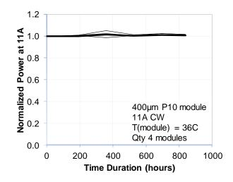
Figure 10: Accelerated lifetest for modules performed at 36 °C and 11 A driving current.
