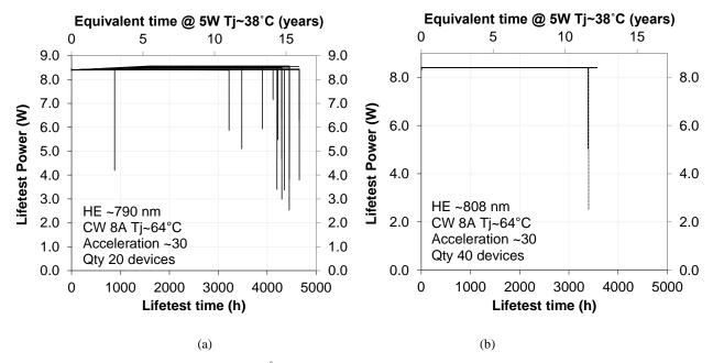
Figure 5: Accelerated lifetest at 8 A and 50 °C heatsink temperature (junction temperature Tj~64 °C on devices with 95 µm stripes and 3.8 mm cavities. (a) 20 790 nm devices, showing facet wear-out after 3000 hours accelerated lifetest, equivalent to >15 year at 5 W 25 °C (b) 40 808 nm devices with two failures observed at 3500 h.
