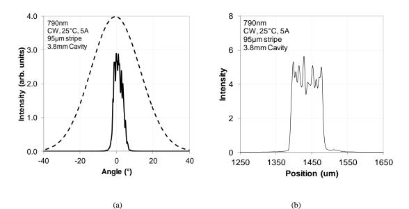
Figure 3: HE 790 nm lasers with 95 μm stripe and 3.8 mm cavity (a) typical fast axis and slow axis far fields operating at 5 A 25 °C (b) typical slow axis near field at 5 A 25 °C
