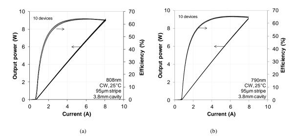
Figure 1: HE Lasers with 95µm stripes and 3.8mm cavities, typical continuous wave (CW) optical power and wallplug efficiency verses drive current operating at 25 °C for (a) 10 808 nm lasers (b) 10 790 nm lasers
