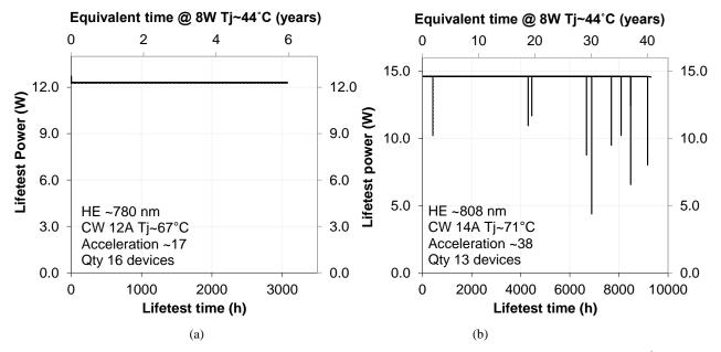
Figure 7: Accelerated lifetest on devices with 200  $\mu$ m stripes and 3.8 mm cavities (a) 16 780 nm devices, at 12 A 50 °C (Tj~67 °C), with no failure and wear-out onset yet (b) 13 808 nm devices, at 14 A 50 °C (Tj~71 °C), tested to wear-out
