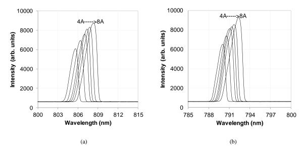
Figure 2: HE Lasers with 95 µm stripes and 3.8 mm cavities, typical spectrum with drive current from 4 A to 8 A operating at 25 °C for (a) 808 nm laser, (b) 790 nm laser
