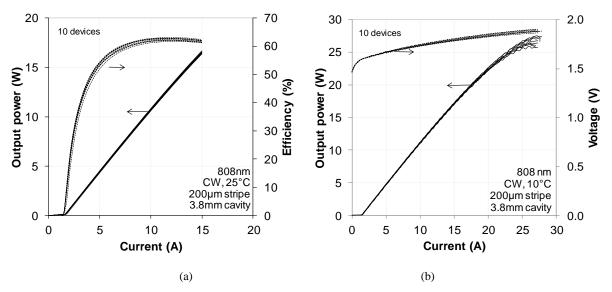
Figure 4: (a) CW LI and efficiency curves of HE structure devices at 25 °C; (b) CW LIV curves of HE structure devices at 10 °C, to power rollover;
