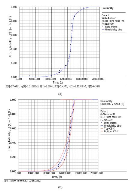
Figure 6: Reliability analysis of lifetests on 95 μm stripes and 3.8 mm cavities, (a) Unreliability using mixed Weibull distribution model (two subgroups), (b) Unreliability with 90% confidence bounds using Generalized Gamma distribution model
