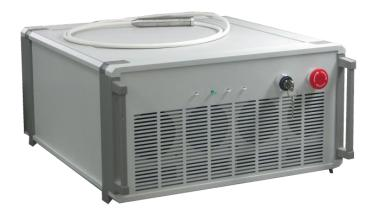
OptoTools CWFL | 100W delivers a highly robust and efficient industrial system for a variety of industrial applications. The air-cooled design delivers a near-diffraction limited beam with WPE up to 25%. The system may be operated in QCW mode as well with modulation frequencies up to 50 kHz.
