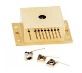
nLIGHT's near-infrared (NIR) single emitter devices, consisting of c-mount and HHL (high-heat-load) packages provide state-of-the-art power and brightness. The small emitting aperture, combined with low beam divergence, make these devices the highest-brightness family of CW diode lasers available in the industry.
