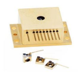
nLIGHT's near-infrared (NIR) single emitter devices, consisting of c-mount and HHL (high-heat-load) packages provide state-of-the-art power and brightness. The small emitting aperture, combined with low beam divergence, make these devices the highest-brightness family of CW diode lasers available in the industry.
