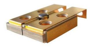
The Summit<sup>™</sup> NL-QD-Q1yzz-L2 Dual Stacked Array packages two conductively cooled diode laser stacks side by side. Each stack is built with up to 6 diode bars (60W QCW to 150W QCW per bar) designed to operate over a broad temperature range.
