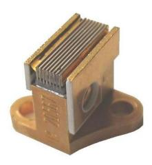
The Summit<sup>TM</sup> NL-QD-Q1yzz-K package is a conductively cooled diode laser stack (of up to 8 bars) designed to operate at very high temperature. This diode laser bar array benefits from the latest advances in technology. It combines the highest efficiency available today with extremely reliable operation at very high junction temperatures.
