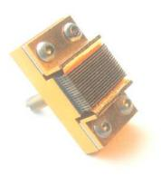
The Summit<sup>™</sup> NL-QD-Q1yzz-G package is a conductively cooled diode laser stack designed to operate at very high temperatures and high QCW optical power. These stacks are built with diode bars of 60W QCW to 200W QCW.
