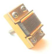
The Summit<sup>™</sup> NL-QD-Q1yzz-G package is a conductively cooled diode laser stack designed to operate at very high temperatures and high QCW optical power. These stacks are built with diode bars of 60W QCW to 200W QCW.
