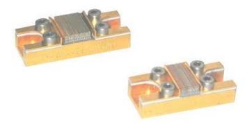
The Summit<sup>™</sup> NL-QD-Q1yzz-B package (up to 10 bars) and NL-QD-Q1yzz-BS package (up to 19 bars) are conductively cooled stacked diode laser arrays designed to operate at very high temperatures. These stacks are built with diode bars of 60W QCW to 200W QCW.
