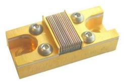
The Summit<sup>™</sup> NL-QD-Q1yzz-B package is a high power diode laser source. The product is based on up to 10 highly efficient 1cm linear bar arrays that are assembled in a stack operating in Quasi-CW mode.
