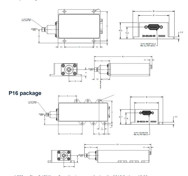
\* 800um fiber 0.13NA configuration increases the length of P10 Package 10.06 mm
