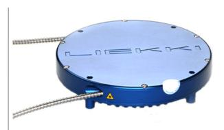
LIEKKI<sup>TM</sup> OE-Yb-L-30 optical engines are plug-and-play CW fiber laser modules for 20 to 30 W average output power laser applications. The optical engines are fully integrated fiber laser subassemblies with signal output and pump input fibers ready for splicing.
