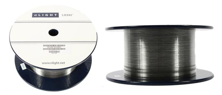
LIEKKI<sup>TM</sup> Yb1200-4/125 fibers are highly doped single mode ytterbium fibers for low-noise, low-nonlinearity preamplifiers and lasers. Their telcom-like geometry makes them compatible with low-cost pump diodes and standard single mode passive fibers. They make an excellent preamplifier in a fiber amplifier chain with double cladding fiber acting as power amplifier.
