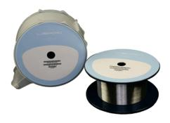
LIEKKI<sup>TM</sup> Yb1200-20/400 fibers are highly doped fibers for medium power fiber lasers and amplifiers. They combine a large core with excellent beam quality and 400 μm cladding capable of accepting medium pump powers.
