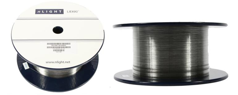
LIEKKI<sup>TM</sup> Yb1200-12/250 fibers are highly doped fibers for medium power fiber laser and amplifier applications. The combination of a single mode core and 250µm diameter cladding makes it ideal for compact medium power fiber laser resonators.
