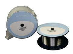
LIEKKI<sup>IM</sup> passive fibers are especially designed and manufactured to match with commercially available large mode area active fibers such as LIEKKI<sup>TM</sup> Yb1200 product line LMA fibers. The passive fibers are matched to the core diameters and numerical apertures of the active counterparts so that excellent beam quality is maintained throughout the fiber laser or amplifier.
