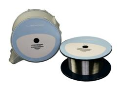
LIEKKI<sup>TM</sup> Er60-20/125, Er60-40/250, and Er60-65/400 fibers are large mode area erbium doped fibers suitable for medium power amplifiers and lasers. These fibers are ideally suited for compact, eye-safe devices (1.55 - 1.6 μm region). Both 980 nm and 1480 nm pump diodes may be used for pump sources.
