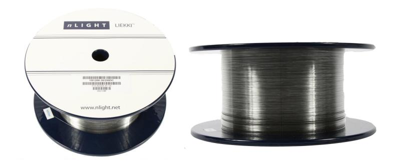
LIEKKI<sup>TM</sup> Er120-20/125 fibers are large mode area erbium doped fibers suitable for medium power amplifiers and lasers. These fibers are ideally suited for compact, eye-safe devices (1.55 - 1.6 μm region). Both 980 nm and 1480 nm pump diodes may be used for pump sources.
