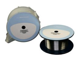
LIEKKI<sup>TM</sup> passive fibers are especially designed and manufactured to match with commercially available large mode area active fibers such as LIEKKI<sup>TM</sup> Yb1200 product line LMA fibers. The passive fibers are matched to the core diameters and numerical apertures of the active counterparts so that excellent beam quality is maintained throughout the fiber laser or amplifier.
