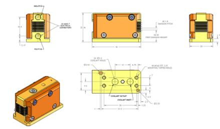
Cascades<sup>™</sup> Vertical Stacked Arrays 10 bar, lensed
