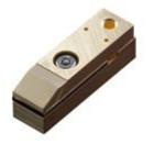
*n*LIGHT's Cascades<sup>TM</sup>, an actively, water-cooled, low thermal resistance bar provides end users with state-of-the-art power, brightness and reliability. These near-infrared (NIR) 1-cm arrays, based on our proprietary MOCVD structure, offer low beam divergence and narrow spectral bandwidth. Cascades<sup>TM</sup> are available in a wide range of wavelengths between 780 nm to 980 nm, and 1400 nm to 1600 nm.
