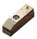
*n*LIGHT's Cascades<sup>™</sup>, an actively, water-cooled, low thermal resistance bar provides end users with state-of-the-art power, brightness and reliability. These near-infrared (NIR) 1-cm arrays, based on our proprietary MOCVD structure, offer low beam divergence and narrow spectral bandwidth. Cascades<sup>™</sup> are available in a wide range of wavelengths between 780 nm to 980 nm, and 1400 nm to 1600 nm.
