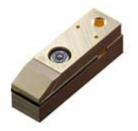
nLIGHT's Cascades<sup>™</sup>, an actively, water-cooled, low thermal resistance bar provides end users with state-of-the-art power, brightness and reliability. These near-infrared (NIR) 1-cm arrays, based on our proprietary MOCVD structure, offer low beam divergence and narrow spectral bandwidth. Cascades<sup>™</sup> are available in a wide range of wavelengths between 780 nm to 980 nm, and 1400 nm to 1600 nm.
