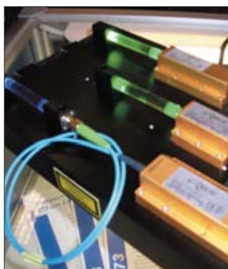
Oxxius' SLIM range now includes 473, 532 and 561 nm DPSS sources. The firm hopes to release a 355 nm version in the third quarter of 2006.
