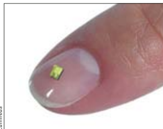
The Luxeon K2 is quoted as having a maximum allowable drive current of 1500 mA and a thermal resistance of 9 °C/W. The PWT1 measures 2 \times 1.6 \times 0.7 mm.
