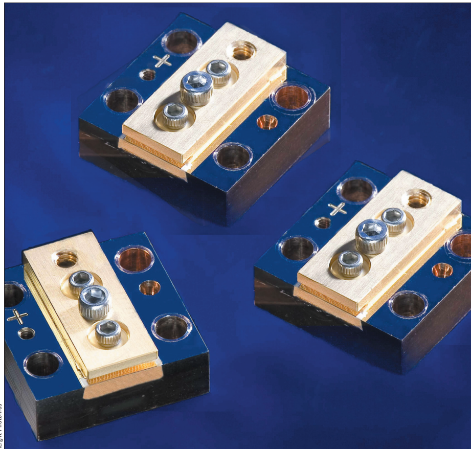
CS mount package for a laser-diode bar: the 1 cm-long bar is attached to a heatsink to remove waste heat and the package measures around 1 × 1 × 0.25 inches (above). A timeline of the affordability and output power of 1 cm laser-diode bar (below). Improvements have enabled the devices to become industrial tools.
