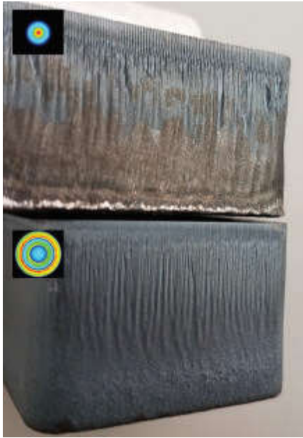
FIGURE 3. A comparison of oxygen-assisted cutting of 1 in. mild steel with a standard 4 kW fiber laser (a) and a 4 kW Corona fiber laser (b) are shown; with the Corona fiber laser, the roughness is lower by a factor of three, the edge is significantly straighter, and the perpendicularity is greatly improved. The Corona fiber laser provides consistent drop performance, whereas the conventional fiber laser does not because of slag on the bottom edge of the part and a concave edge shape.
