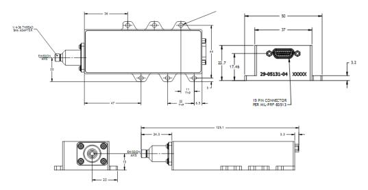
\* 800um fiber 0.13NA configuration increases the length of P10 Package 10.06 mm
