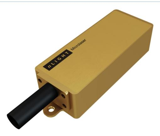
nLIGHT's DPSS 1064nm Microlaser M20 is designed with integrated output optics, thermal control and a complete electronics package for a wide range of applications. Pumped with nLIGHT's patented nXLT diodes, the Microlaser M20 offers exceptional beam quality and high pulse energy from a compact package.
